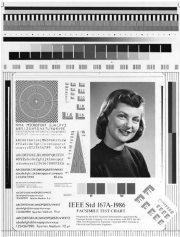
**Fig. 5 - CCITT fax test chart 167A, 1986.**
